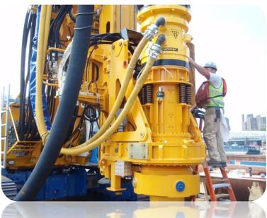
For maximum production in harder rock drilling, experienced drillers turn to Reverse Circulation "RC" Methods. Reverse Circulation ensures continual removal of cuttings that can be controlled to meet environmental constraints. Bermingham has developed its RC Swivel to enable clients to utilize this advanced drilling technique using their existing drilling rig. The Bermingham RC attachment can fit any configuration required.
