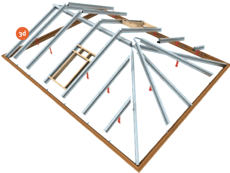
Temporary fix remaining rafters including any pre-engineered window framing (if required).
