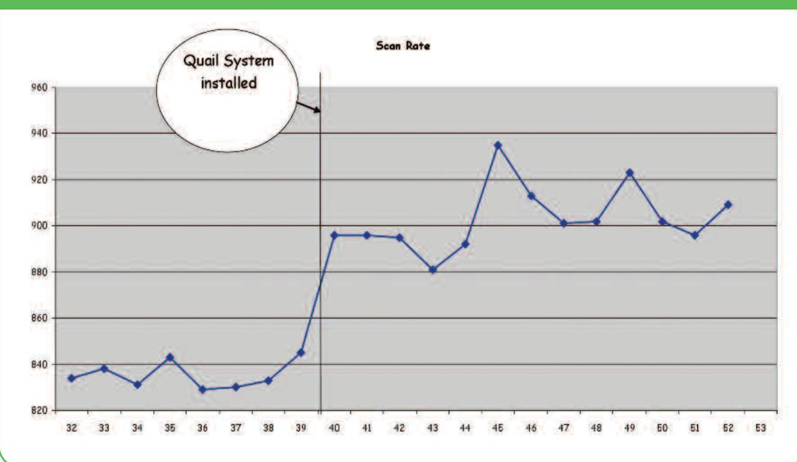
**Tables 4 and 5** show results from another large-scale supermarket chain which wanted to measure the impact of using **Quail Digital Headset System** with Messaging Keypads at their tills when measured against scan rate and through put. If headsets improved productivity against a constant throughput then there was the possibility of requiring fewer tills to be operational.
