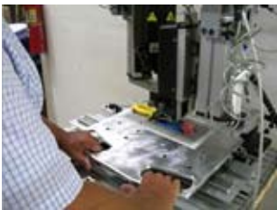
The R9's movable jig allows for absolute positioning of any Elastic Staple
