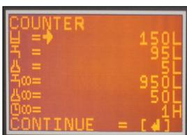
The operation counter warns before the container is empty and provides information concerning the used water and concentrate data as cycle and total counter.
