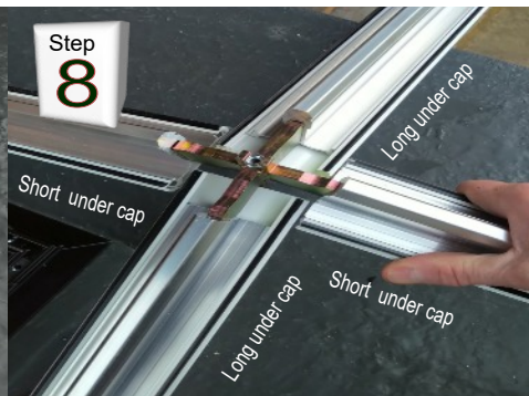
Push rafters on to spider. Long cap under facing long cap
