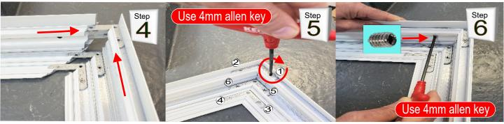
Join the frames on a flat surface. Tighten each ratchet cleat in order Once mitres are tight, lock in place shown, 1 & 2 being first. with grub screw shown.
