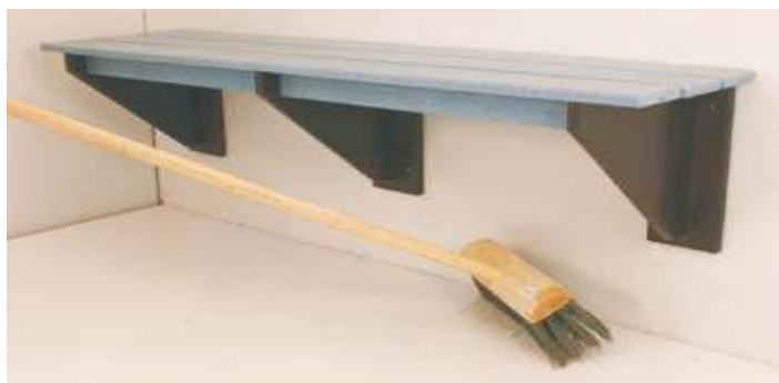
Bench Tops are one piece, & slotted for drainage. Each Bracket requires 3 Wall Anchors. Each bracket is fixed @ 450mm Centres approx.
