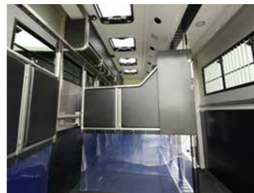
The ramp comes with a rubber cover and integrated horizontal slats. The side panels provide for extra safety when loading or unloading the horses.
