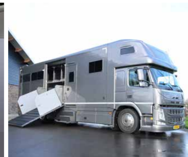
A hinge at the centre of the partition makes it easily foldable which facilitates loading and unloading the horse via the side tailgates.
