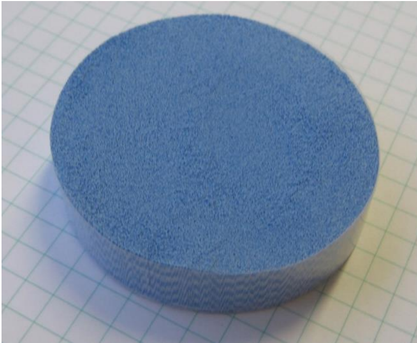
Fig. 4.1: Cut filament puck (out of the filament hank)
