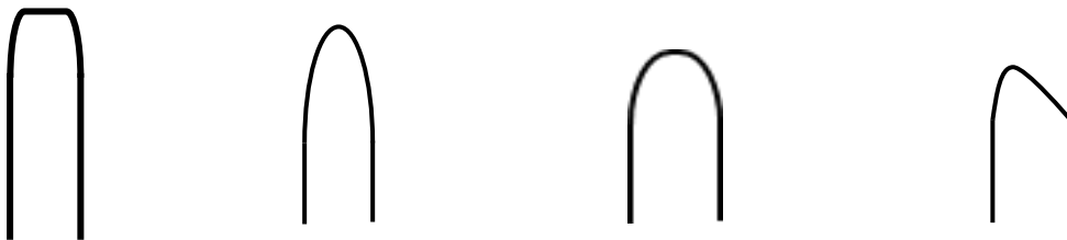
Fig. 7.1: Flat end tip Fig. 7.2: Pointed end tip Fig. 7.3: Half dome end tip Fig. 7.4: Non-symmetric tip
