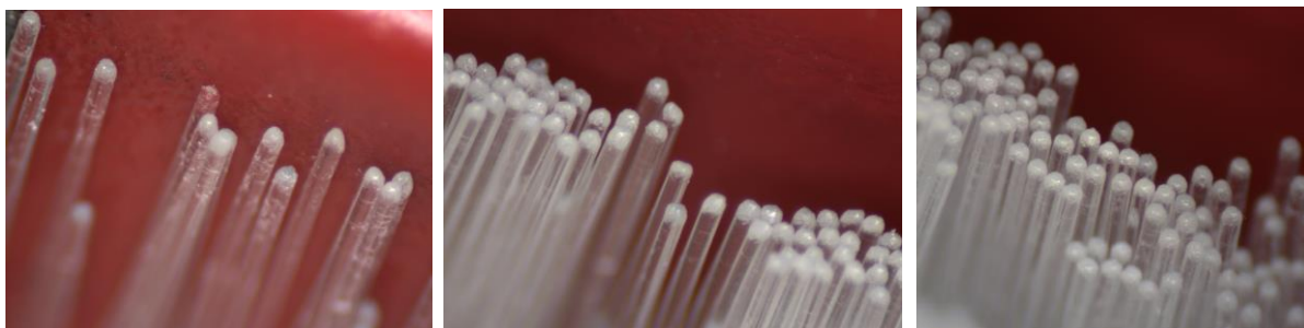
Fig. 6.5: Magnified tips (end-rounding quality)
