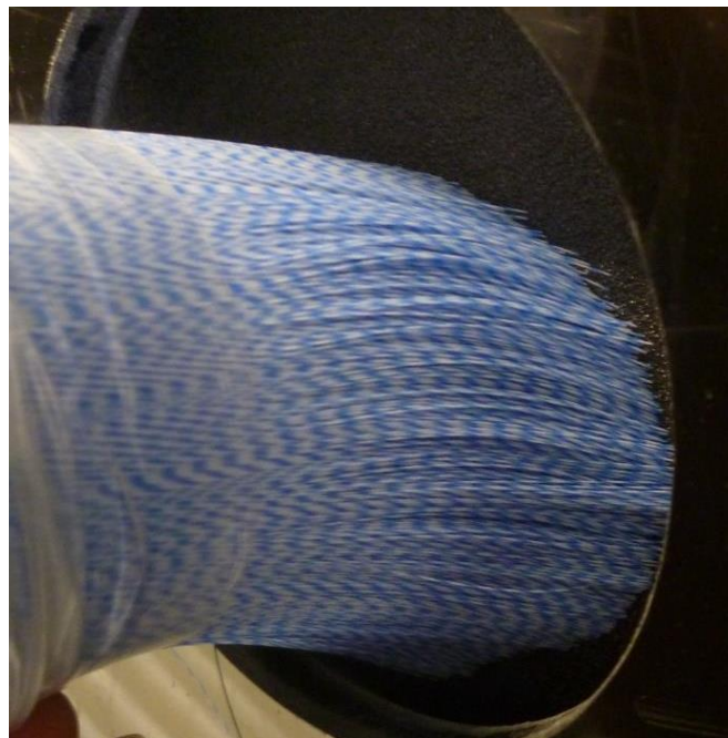
Fig. 4.6: Loosened filaments out of the hank during grinding procedure.
