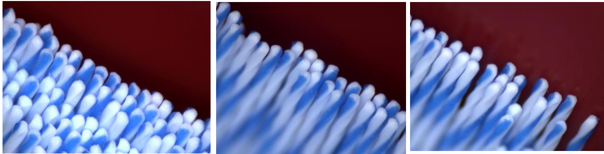
Fig. 6.3: Magnified tips (end-rounding quality)
